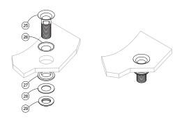
Insert drain rim (25) into the basin placing the Teflon washer (26) under the rim. From below slip on washer (27) onto the bottom thread of the drain rim and secure to basin with drain nut and washer (28 and 29).
