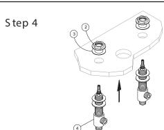
Remove top fastening nut and washer (2 & 3) from the lavatory valve. (NOTE A: All lever handle sets are supplied with one right-hand valve and one left-hand valve. Install valve with the blue dot on the cold side. Insert valve from below through hole in lavatory or counter-top.
