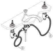
Connect stainless steel flex lines (6) from valve outlets to spout tee (10). Flex lines should be looped as shown indiagram. FLEX LINES MUST NOT BE KINKED.
