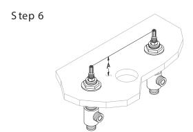
Set valve to proper rough-in height "A", by adjusting bottom-fastening nut. Secure valve by tightening top fastening nut \*YOU MAY NEED TO CUT THE ALL BROACHED STEM TO REDUCE THE VISIBILITY BETWEEN HANDLE AND ESCUTCHEON. Repeat procedure for the second lavatory valve. Please see page P99030A for the "A" measurement for your trim.
