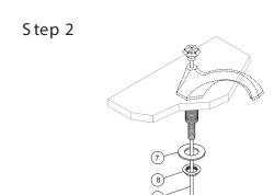
Insert spout base nipple into center hole in lavatory or counter top. Install stainless washer (7) and spont (8) on spout nipple and tighten. Place pop-up knob rod (14) though spout.
